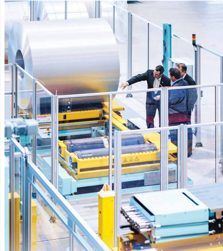
▲ In modern car manufacturing, as with this Schuler laser blanking line at the Mercedes-Benz plant in Kuppenheim, thousands of high-strength, weight-optimized car body parts are blanked every day out of extremely heavy aluminum coils.
