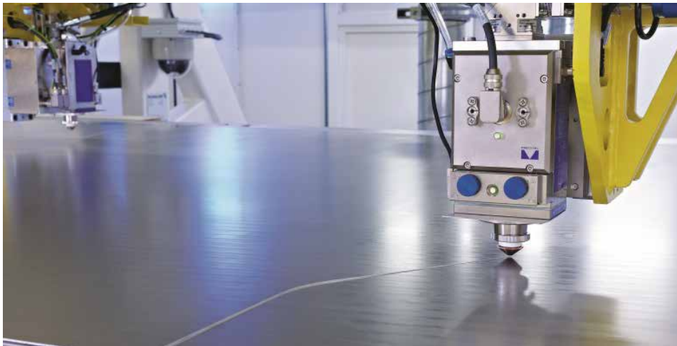
▲ As the Schuler line uses fiber lasers, no dies are required – in contrast to conventional blanking lines.
