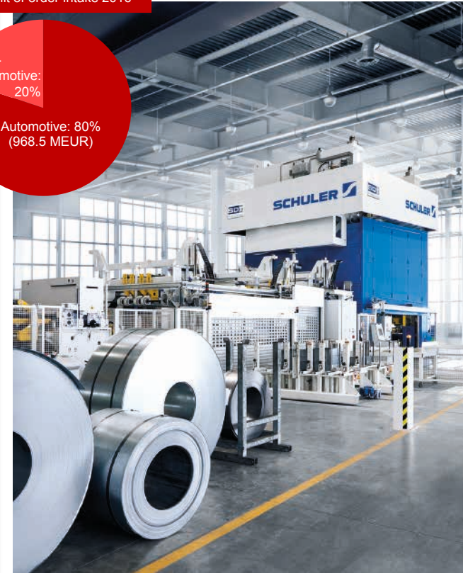
▲ Production of double parts at an automotive components supplier with a servo press in tie rod design with 16,000 kN press force
