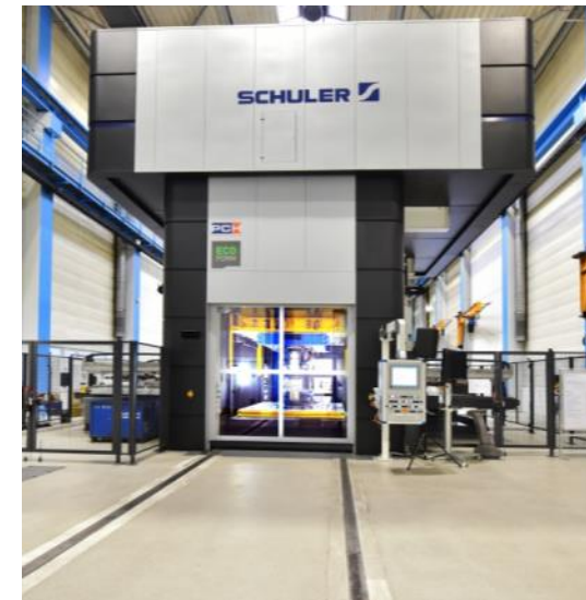
▲ Hydraulic hot stamping line with PCHflex technology
